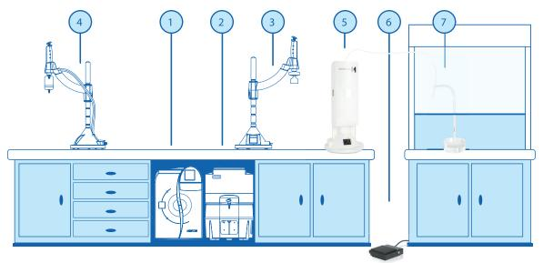
1. Milli-Q<sup>®</sup> Integral water purification system purifies tap water to pure (Type II) and ultrapure (Type I) water. Designed for bench integration to save laboratory space; patented Merck Millipore Elix<sup>®</sup> technology minimizes operating costs.
